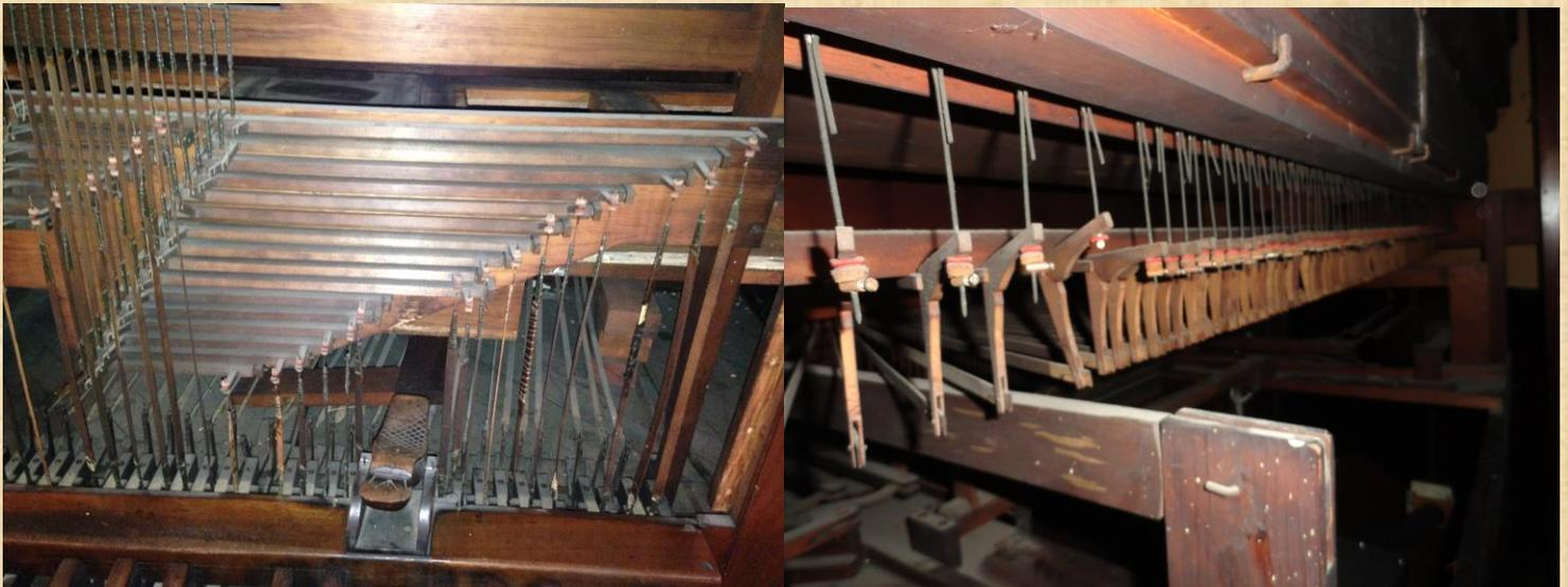
Seen here is some of the mechanism of our pipe organ, when it was opened up for its restoration. Called tracker action, it has been largely replaced with direct electric action or electro-pneumatic action in the 20<sup>th</sup> century, though it has enjoyed something of a revival in recent years due to the old system's better responsiveness to an organist's touch.
